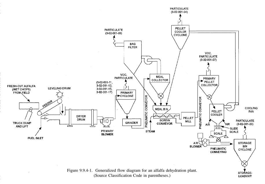
Lesser emission sources include the downstream cyclone separators and the bagging and loading operations.
