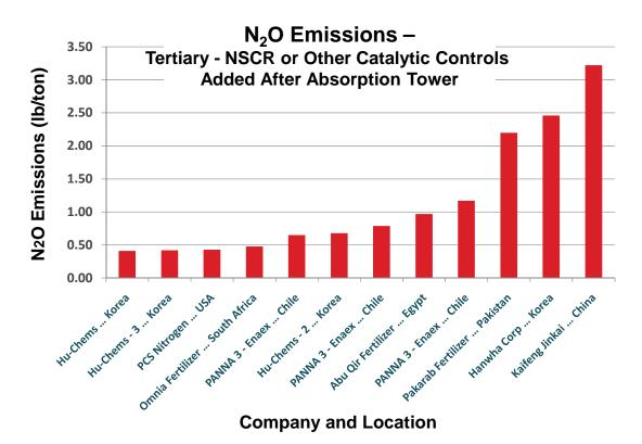
Figure 8. N<sub>2</sub>O emissions from Tertiary Controls
