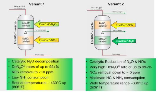
**Figure 6– Uhde Combination N<sub>2</sub>O and NO<sub>X</sub> Control for Nitric Acid Production Plants** Source: ICAC, 2009.
