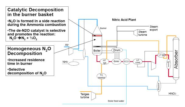
Figure 4 – Yara Secondary N<sub>2</sub>O Control from Nitric Acid Production
